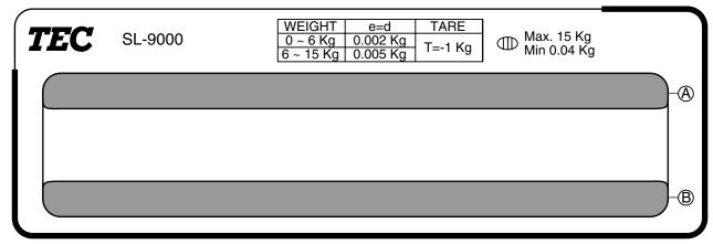
For the QR machine, the following multi-linqual display stickers are provided to adapt machines to use in various countries. Select one of them and affix it to positions (A) and (B) on the remote display. (Refer to Section 7 How to affix the remote display sheet.)
